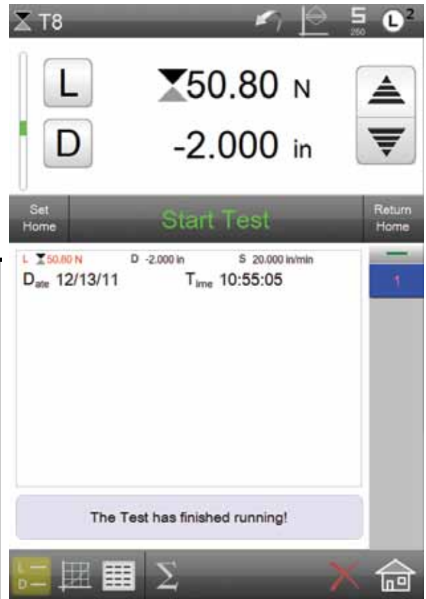
The L result is less than the Tolerance range, therefore, the result is a “failed” result. The coefficient is displayed in RED to indicate a failed result.
