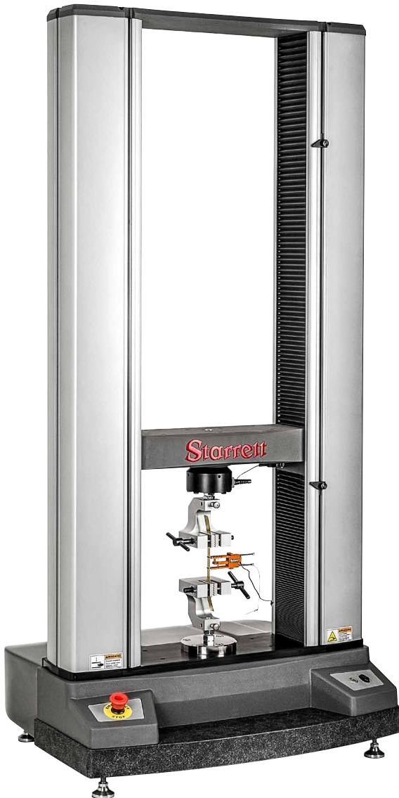
MMD-50K Series Testing Frame (50kN, 5000 Kgf, 11,250 lbf)
