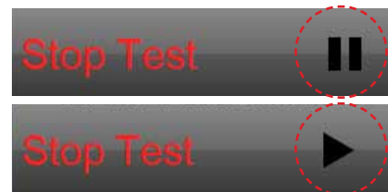
Start/Pause/Stop Test Soft Targets on Controller View Pause is available since an Extensometer is being used
