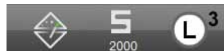
L3 Extensometer Indicator Not displayed when extensometer is not connected to test frame
