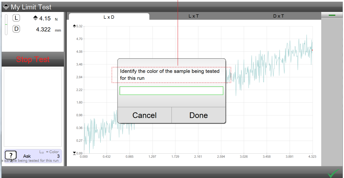
L2 Plus Test An ASK prompt is displayed requiring the operator to answer
