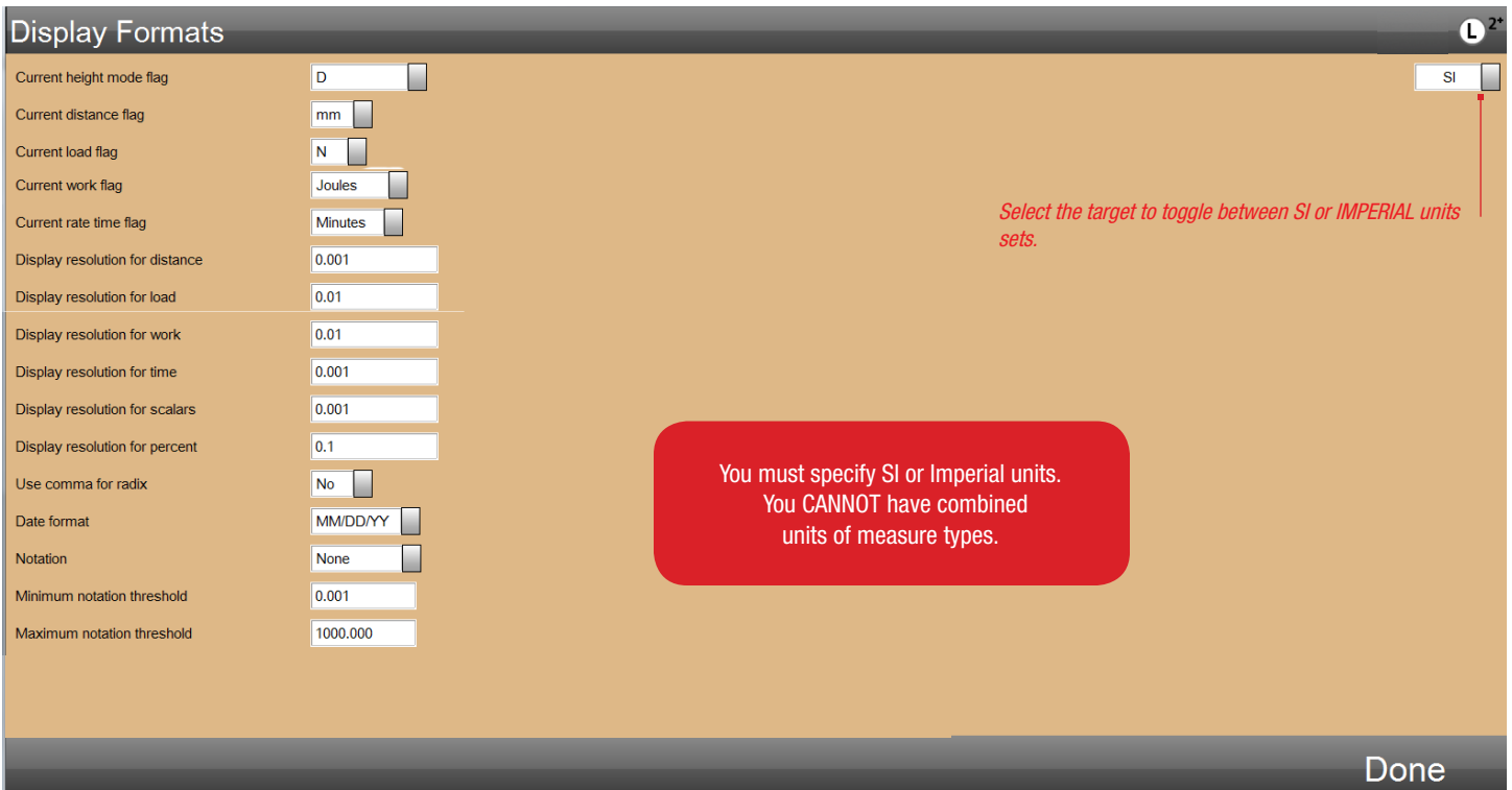
L2 Plus Test Builder - DISPLAY FORMATS Use to specify global unit of measure sets, units and other display formats
