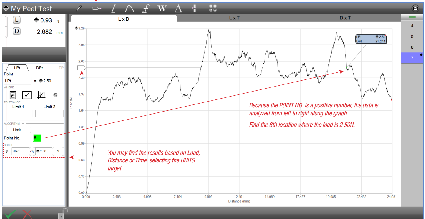
L3 Point Limit Measurement Find the 8th location on the trace where the load value is 2.50N
