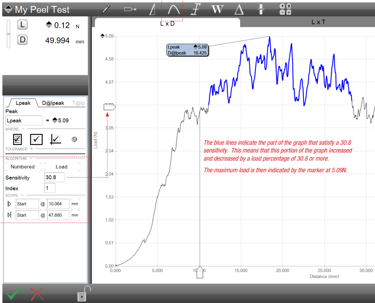
L3 Peak Measurement on an adhesive test
