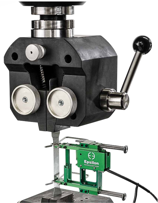
L3 Test Builder - Sample Definition Step An Epsilon Extensometer used on an L3 System
