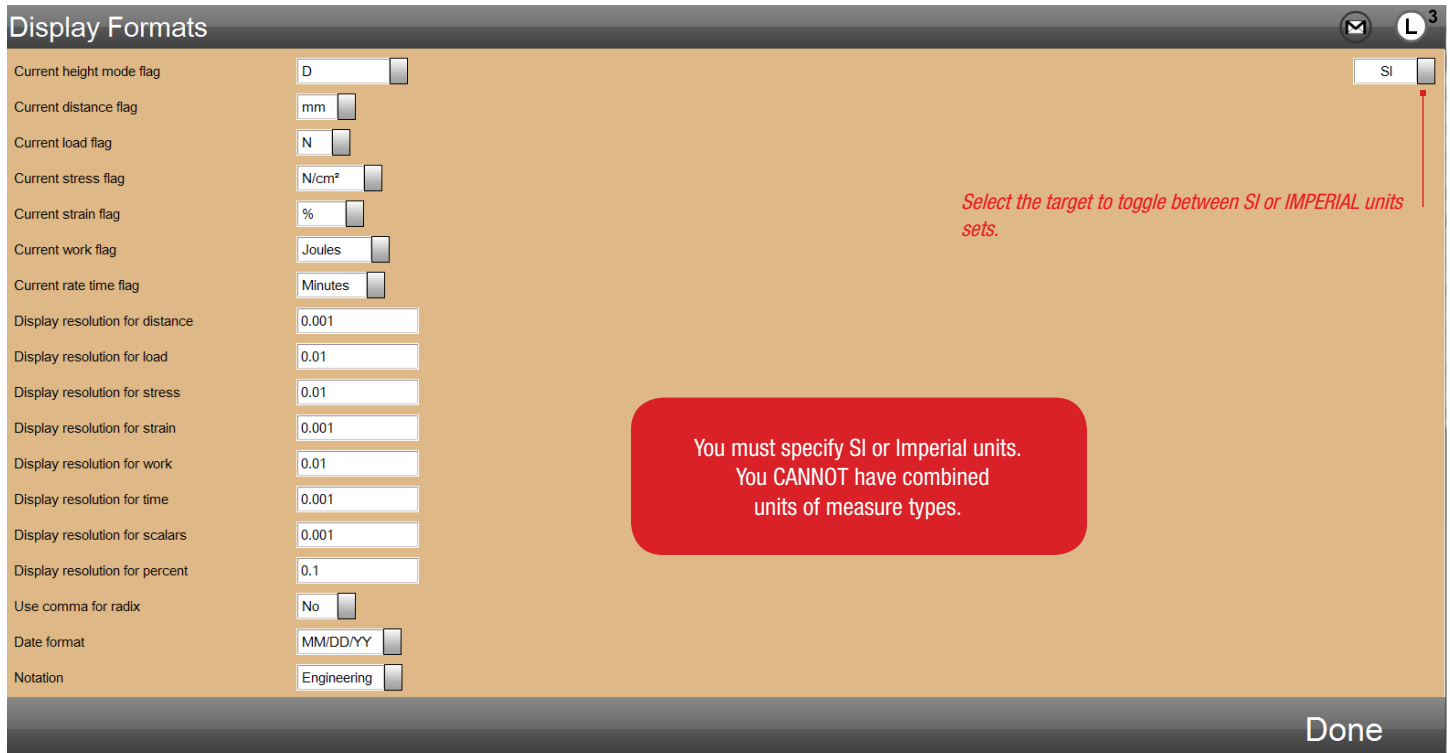
L3 Test Builder - DISPLAY FORMATS Use to specify global unit of measure sets, units and other display formats
