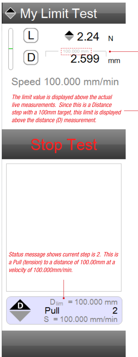
Controller view during active test run Displays status message of current Step 2
