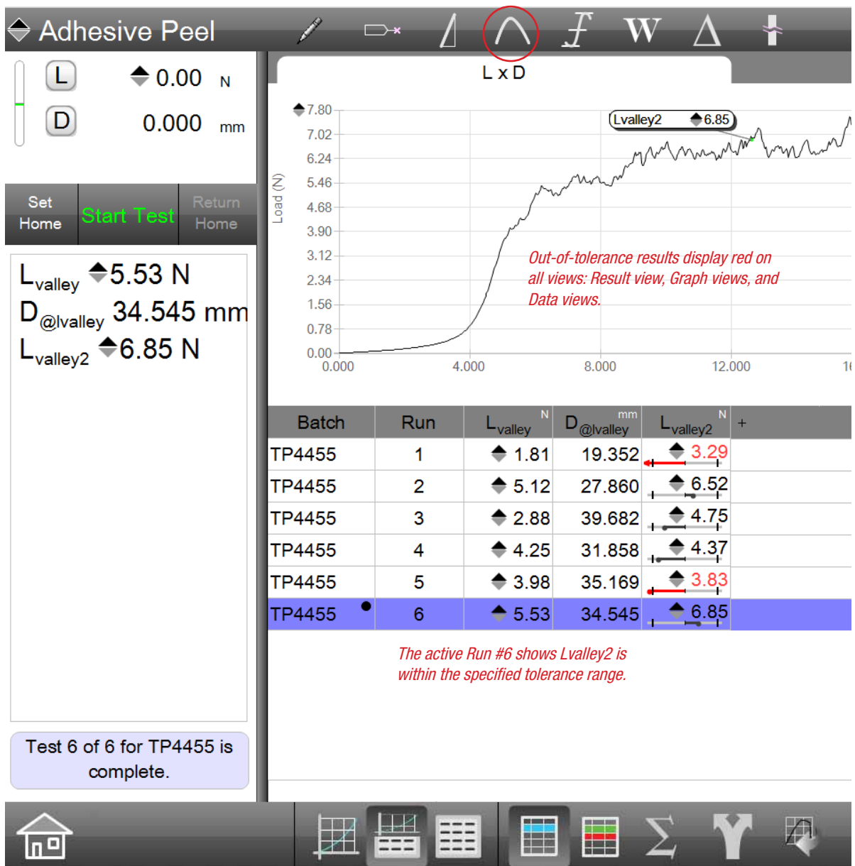
Maximum Valley with Tolerance Out-of-tolerance results display in red text
