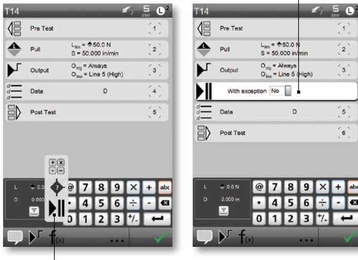
Select an END step within your conditional branching sequence to end the sequence should an exception occur.
