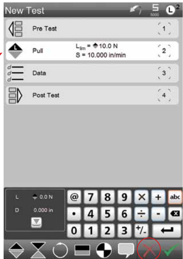
Select the Stage Move to Delete. Select the "X" to delete the step.
