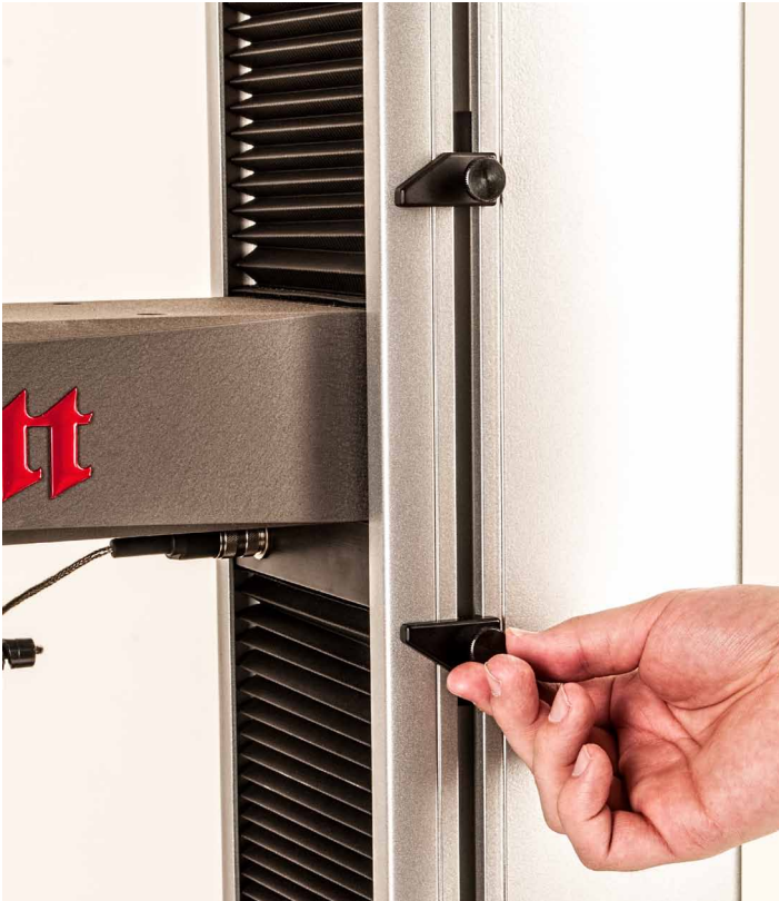
MMD /FMD Series Crosshead Travel Limits
