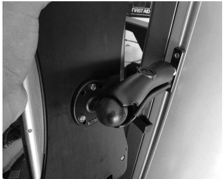
Fix spring clip onto both balls and tighten
