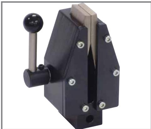
The test fixture is secured to the Clevis adapter using a 8mm grip pin.
