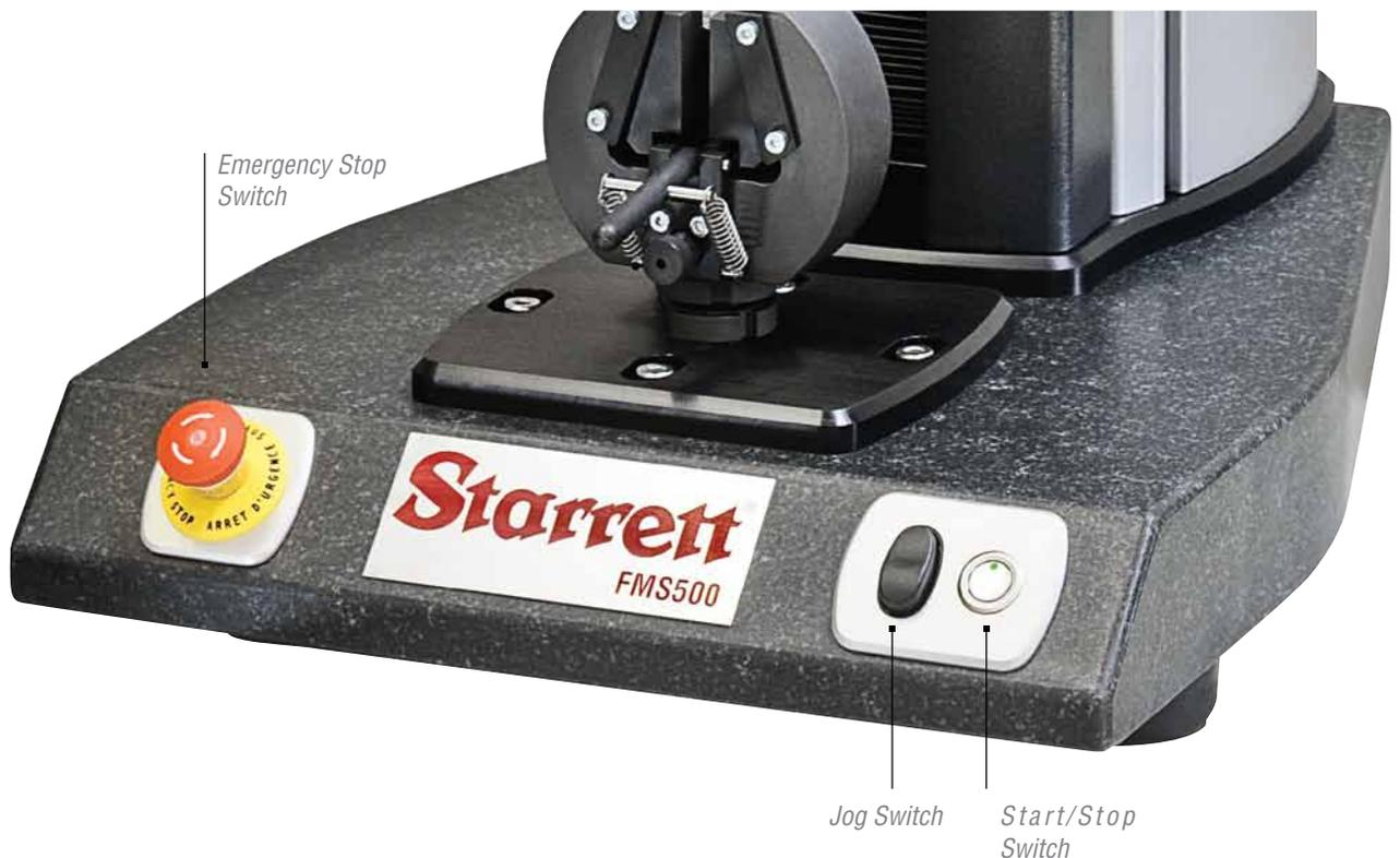
JOG UP - press the up portion of the switch to cause the crosshead to move upward. Release the switch to stop motion.
