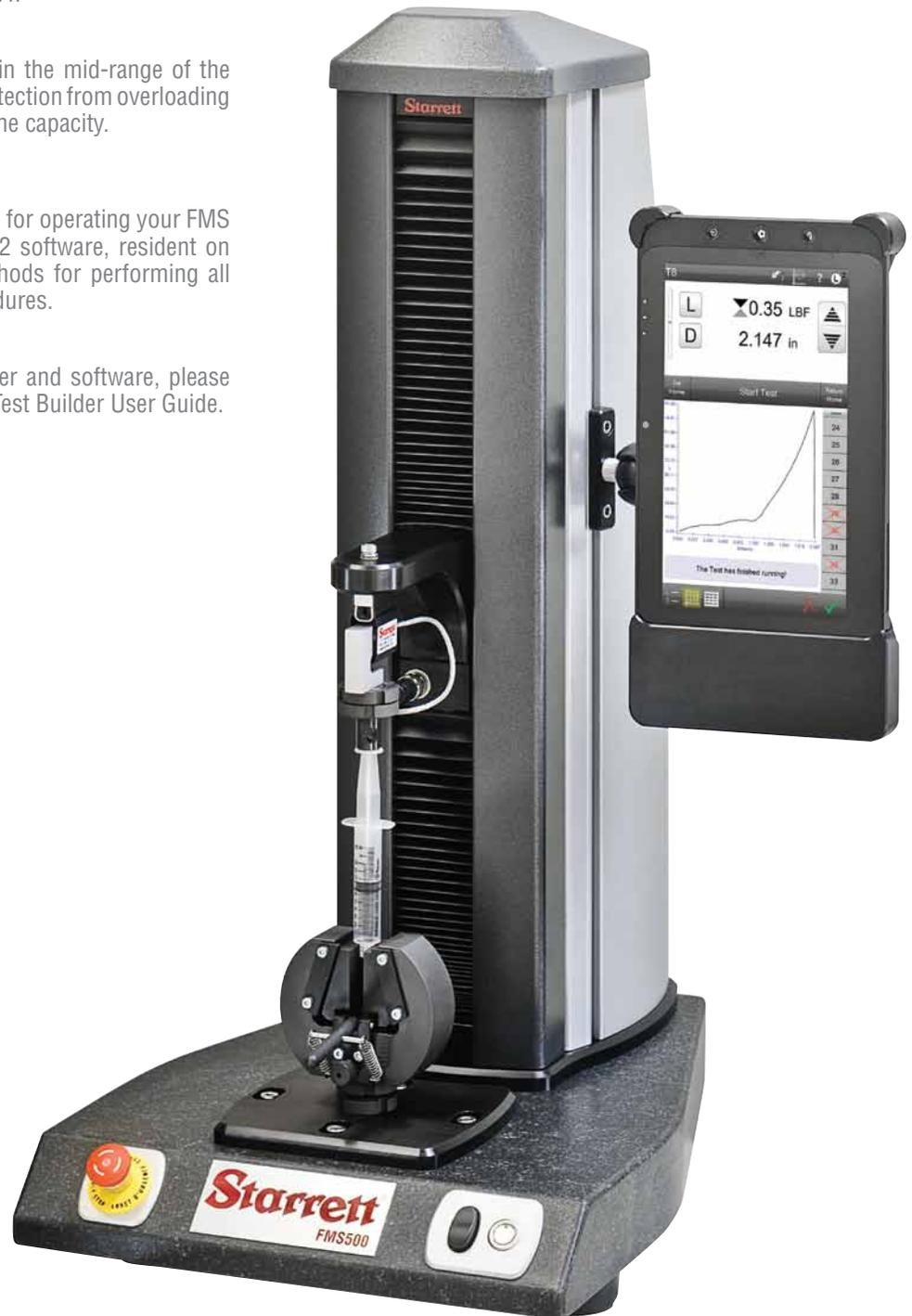
FMS500 Series with L2 Controller and optional Load Cell Sensor and Wedge-action Test Fixture
