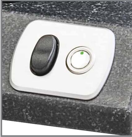
Use the START/STOP Switch to start or stop a test. An LED on the START/STOP Switch illuminates to show that a test is in progress or that the tester is ready to perform a test.
