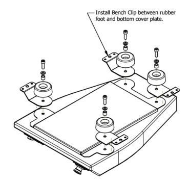
Remove the mounting feet on your FMS frame and insert a mounting clip onto each foot. Re-thread the mounting feet into the base. Use all four mounting clips to properly affix the machine to the surface.
