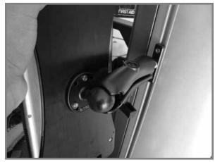
with a ball joint. The L2 Controller attaches to a plate with a ball joint. An adjustable RAM arm attaches to both ball joints. The RAM arm lets you position the L2 Controller for maximum comfort and easy operation.
