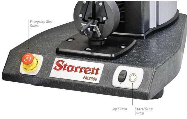
JOG UP - press the up portion of the switch to cause the crosshead to move upward. Release the switch to stop motion.
