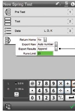
When Append is used, a new row in the file is added when a test run is completed.
